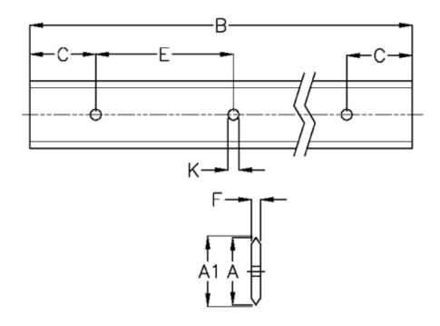
$\begin{array}{lll} A & = 76 \\ A1 & = 76.81 \\ B & = 2336 \\ C & = 43.0 \\ E & = 90 \\ F & = 9.12 \\ For bearing = J54 \end{array}$
